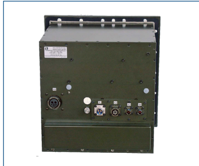
Rear View: Box with 80 A power-connector (left) and signal connectors
